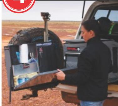
The kitchen bench is opened and secured to the fridge slide with locating pin and bracket.
