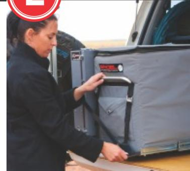
The fridge slide is unlocked, and both fridge and kitchen slide out together easily on the piranha heavy duty runners.
